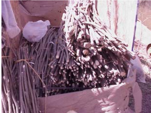
A shipment of live stakes for a streambank restoration project
